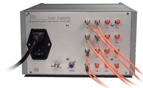
Fiber optic connectors of the ATTanalyzer
